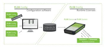
The configuration software on the PC (e.g. FL3X Config Basic) generates a configuration file for the end device.
